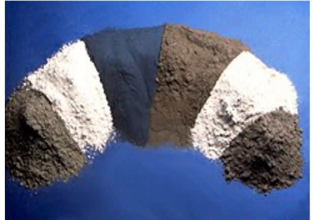
Supplementary cementing materials. L-R: Fly ash (Type CI), metakaolin (calcined clay), silica fume, fly ash (Type F), Slag, and calcined shale.
