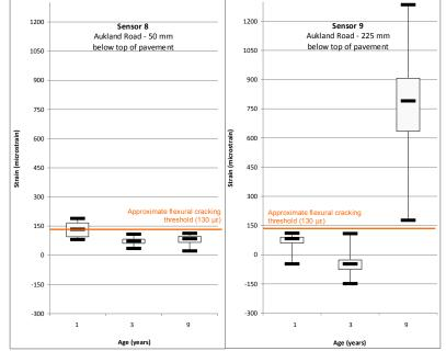
FIGURE 7 Comparison of strains in JPCP after 1, 3 and 9 years of service.
