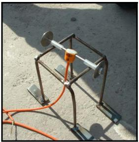
FIGURE 4 Typical strain gauge installation before paving.
