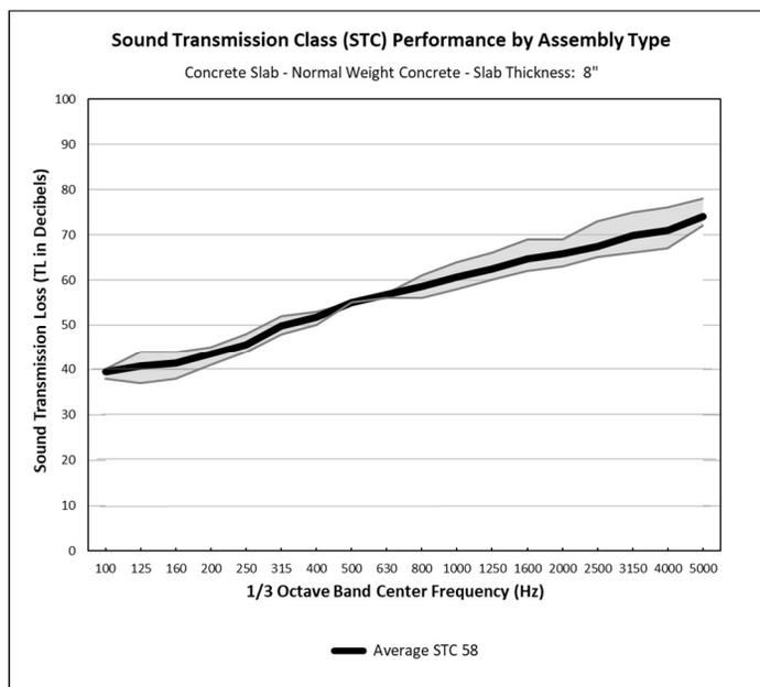
FIGURE 2. Concrete Floor-Ceiling Assemblies – Acoustics Performance Interactive Graph
