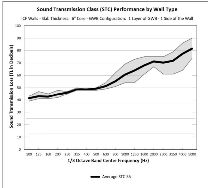
FIGURE 3. Concrete Wall Assemblies – Acoustics Performance Interactive Graph
