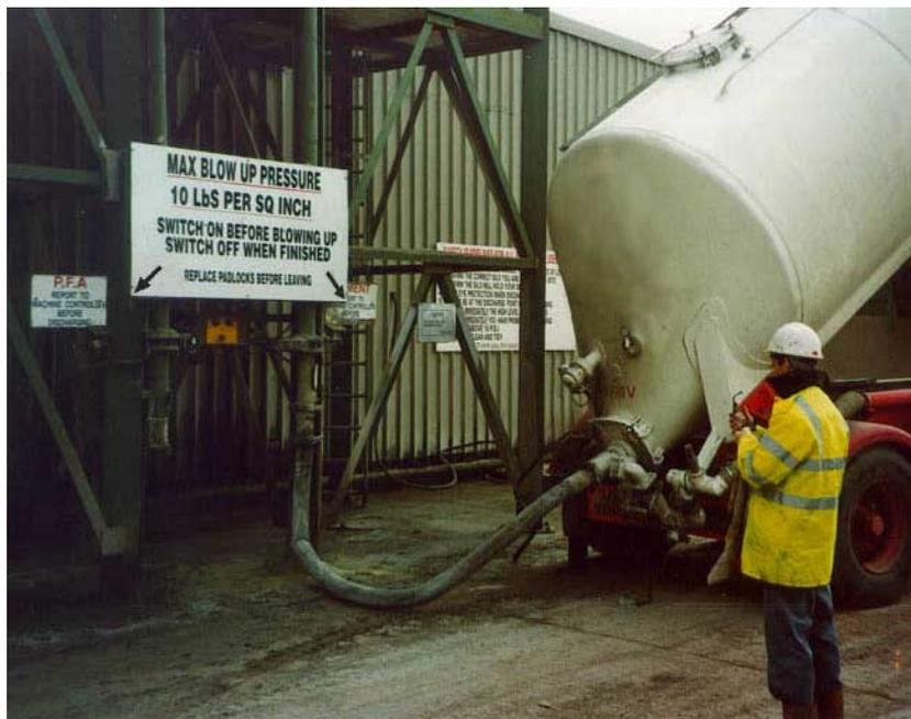
**Figure 6.** Delivery from tipping tanker. Note signs close to delivery point.
