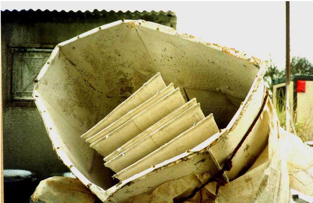
**Figure E1.** Filter housing which has been ejected from the top of a silo. The bolts holding the housing in place have been torn through the metal flange.
