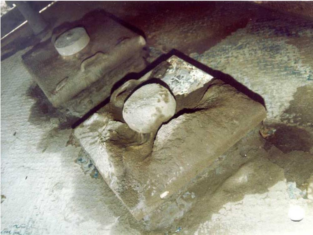
**Figure E2.** Poorly maintained PRVs. The build up of cement powder around the PRV indicates a lack of maintenance and incorrect operation. The PRV should only lift in an emergency, whereas the one pictured above appears to have been routinely lifting during delivery, resulting in the observed accumulation of powder.
